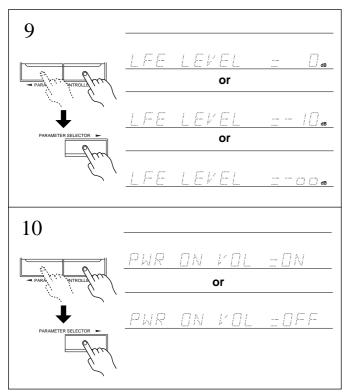
9. Press the PARAMETER SELECTOR► button to display the LFE LEVEL parameter, and press the PARAMETER CONTROLLER
